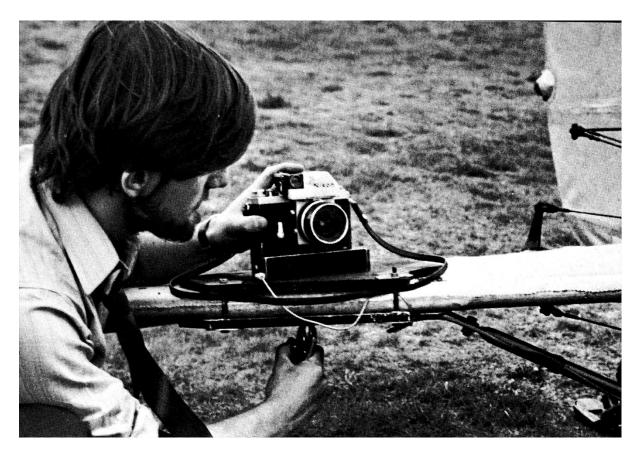
I bolted special plates onto the aircraft's tail to support a remotely fired camera. A long cable draped along the fuselage connected to a microswitch on the pilot's joystick—you can see it trailing along the fuselage—enabling him to take pictures as he dived in on the fleeing man.
